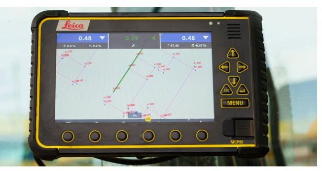
The Leica Viva GS16 GNSS Rover allows Tough Construction to establish control, create coordinate systems and set up base stations to position Excavators and Dozers using Machine Control. The accompanying Leica Captivate software allows data to be viewed and used, providing a clear understanding of data in 2D and 3D views.
